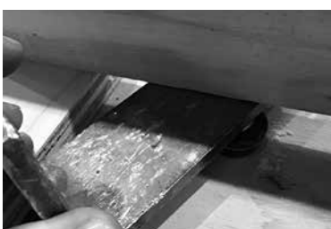
The block can pass through the gap between the anchor pin head and a panel placed on the upper sleepers.
